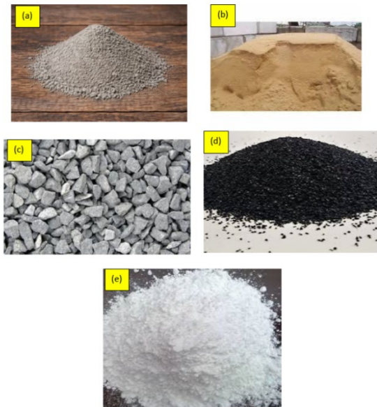
Figure 1. Materials used in the present investigation: (a) Ordinary Portland Cement (43 Grade), (b) Natural River sand, (c) Crushed coarse aggregate, (d) Copper slag, and (e) Eggshell powder
