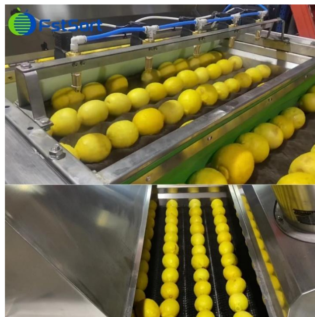
Figure 1. Inline spray system depositing a mist of carnauba-based wax onto oranges before forced-air drying (Vegetablemachines, n.d.)
